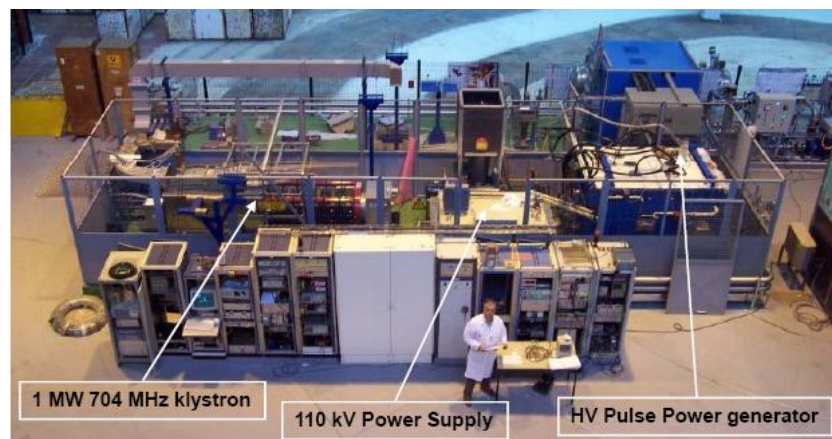
From left, clockwise: the chopper beam line installed at CERN, the 1 MW test stand for superconducting cavities at CEA Saclay, a chopper structure
