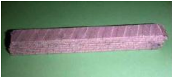
Cable stack with ceramic insulation
