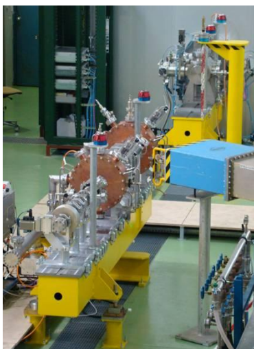
Prototypes of superconducting accelerating structures and components. From left, elliptical cavity B, spoke cavity, prototype coupler.
