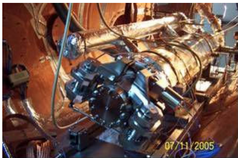
Figure JRA1.10.3: Cold Tuning System (CTS) with Noliac Piezo Tuner mounted on 9-cell cavity for cold test in CryHoLab.
