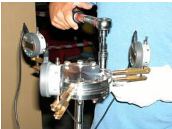
Figure JRA1.2.6: Bolt tightening with torque meter and liquid nitrogen temperature leak test.
