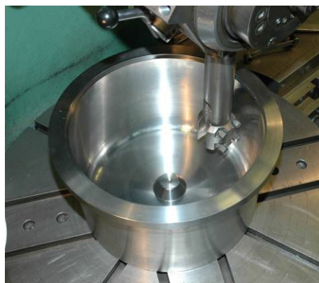
Figure JRA3.2.19: A half tank on a vertical lathe.
