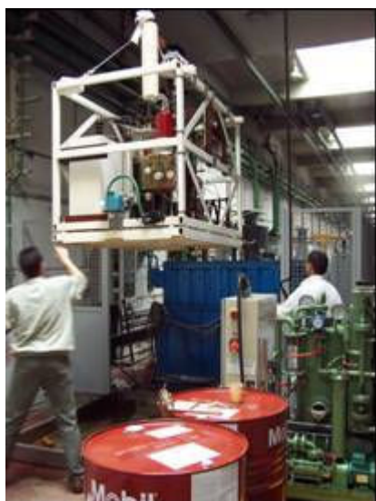
Figure JRA1.10.1: The klystron-modulator components are transferred, after cleaning, in the oil-tank refilled with 4300 liters of new oil.
