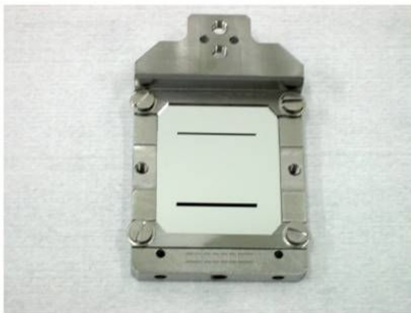
Figure JRA1.11.10: The DR screen with two slits of 0.5 and 1 mm respectively.
