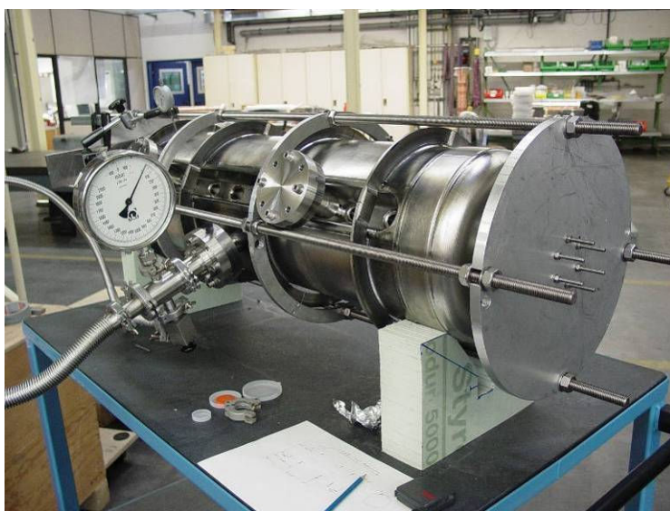
Figure JRA3.3.21: The CH-cavity during a vacuum test before the chemical treatment.
