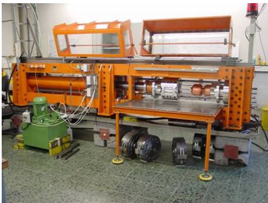
Figure JRA1.3.5: View of the hydroforming machine
