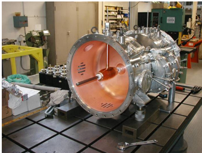
Figure JRA3.2.15: Alignment of the drift tube inside the CCDTL pre-prototype.
