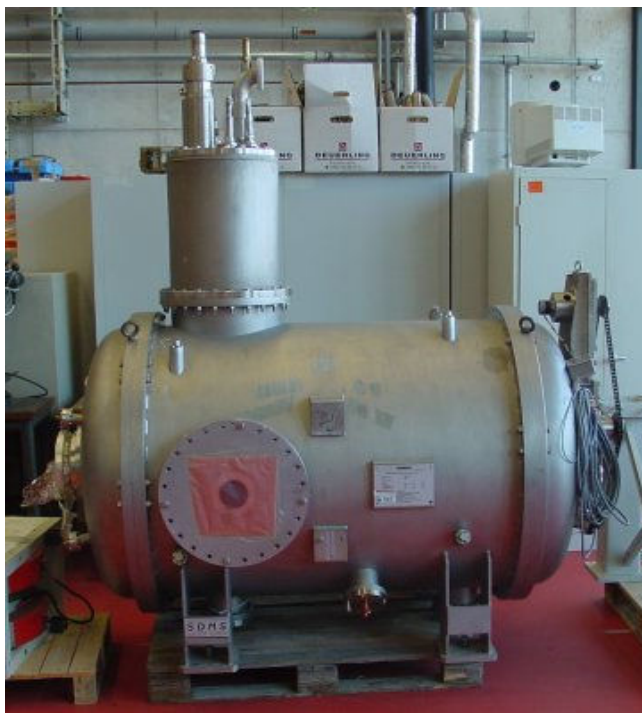
Figure JRA3.3.30. Cryomodule with tuning possibility for operation in horizontal position
