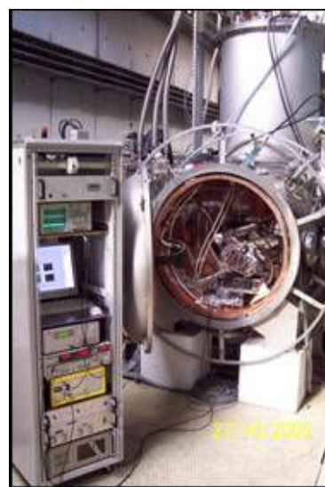
Figure JRA1.10.3: Cold Tuning System (CTS) with Noliac Piezo Tuner mounted on 9-cell cavity for cold test in CryHoLab.
