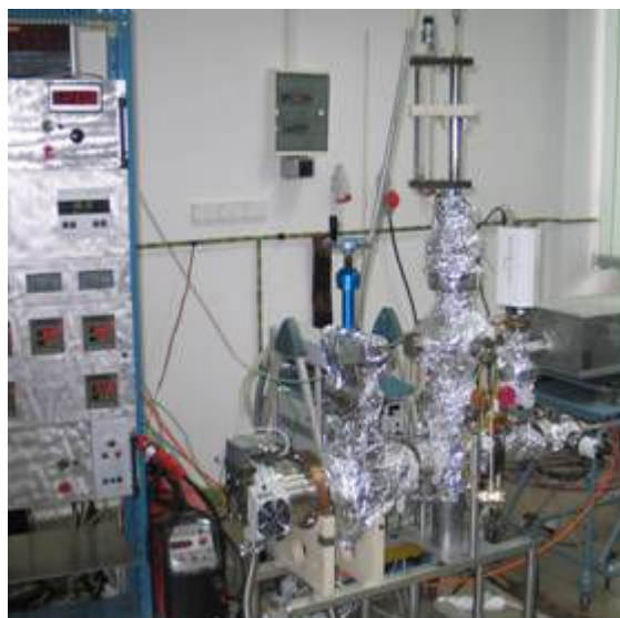
Figure JRA1.4.1: Scheme of the linear-arc UHV system and modified facility at IPJ (Swierk).
