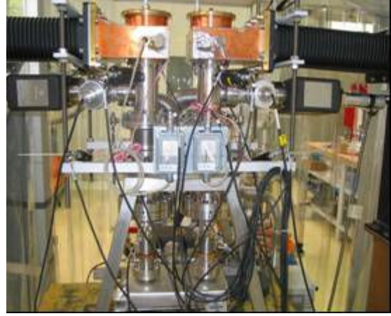
Figure JRA1.7.6: TTF-III couplers being conditioned.
