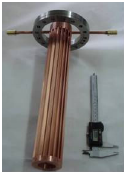
Figure JRA1.4.3: View of the cylindrical Venetian-type micro-droplet filter.
