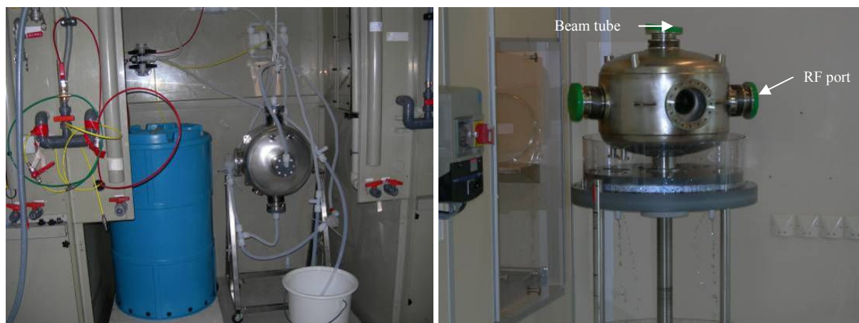
Figure JRA3.3.12: Chemical polishing (left) and Spoke cavity on the HPR set-up (right)
