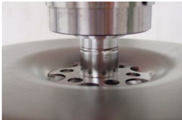
Figure JRA3.3.23: Connection between outer drift tube and cavity body
