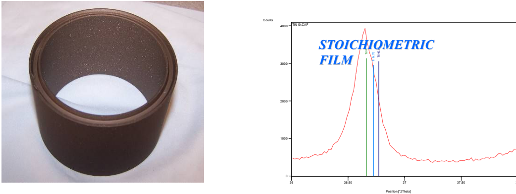
Figure JRA1.7.2: (Left) Tin coated ceramic window, thickness = 800nm. (Right) results of the diffractometry are shown. The film appears to be stoichiometric.
