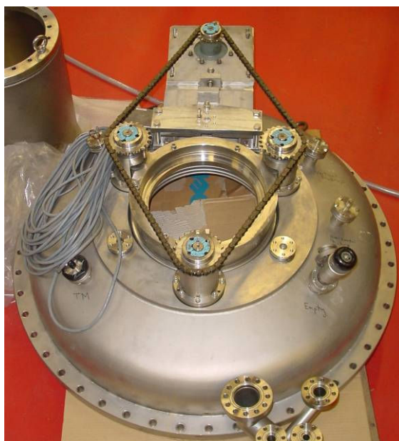
Figure JRA3.3.27: Mechanical tuning unit on one end of the cryostat
