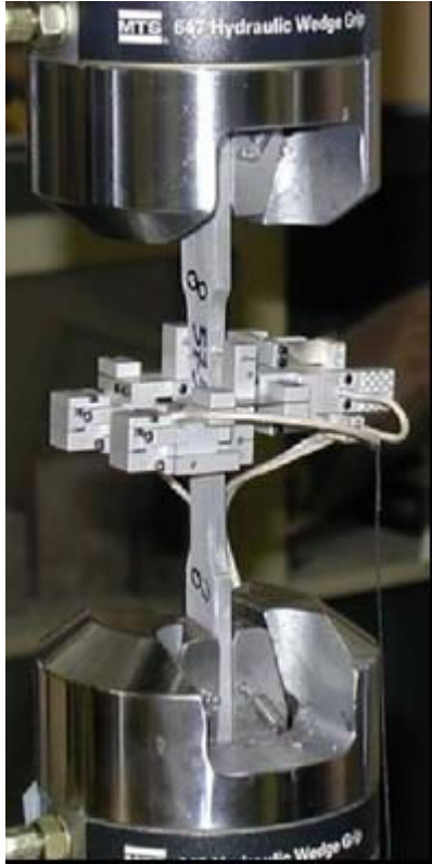
Figure JRA1.2.1: Experimental tensile tests on an Al specimen alloy.
