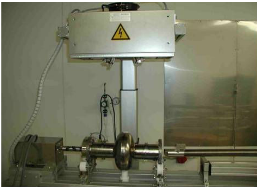
Figure JRA1.5.15: Dry-ice cleaning system with the new IR heater
