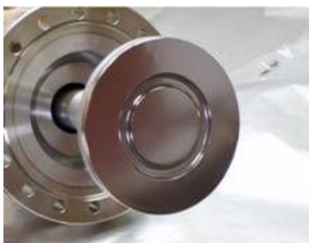
Figure JRA1.4.12: Large copper sample fixed upon an insulating support (just before the coating).
