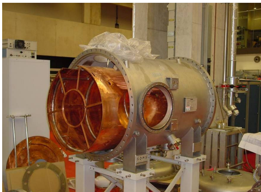
Figure JRA3.3.26: Center part of the vacuum chamber and the copper thermal shield inside
