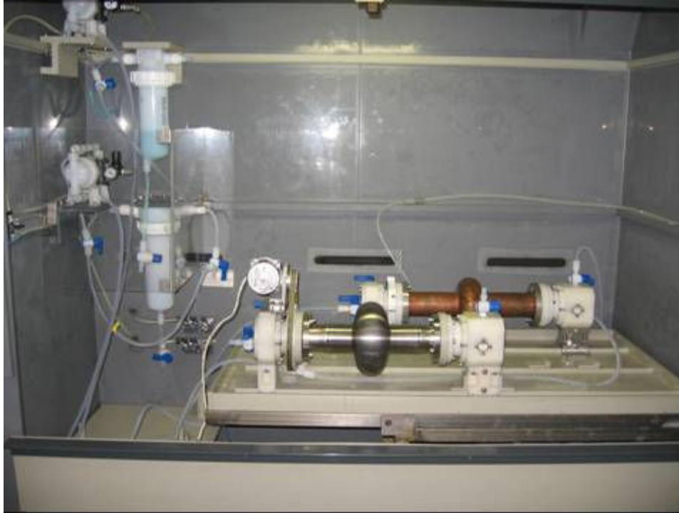
Figure JRA1.5.8: The rotating cavity EP system built for the treatment of both Niobium and Copper.
