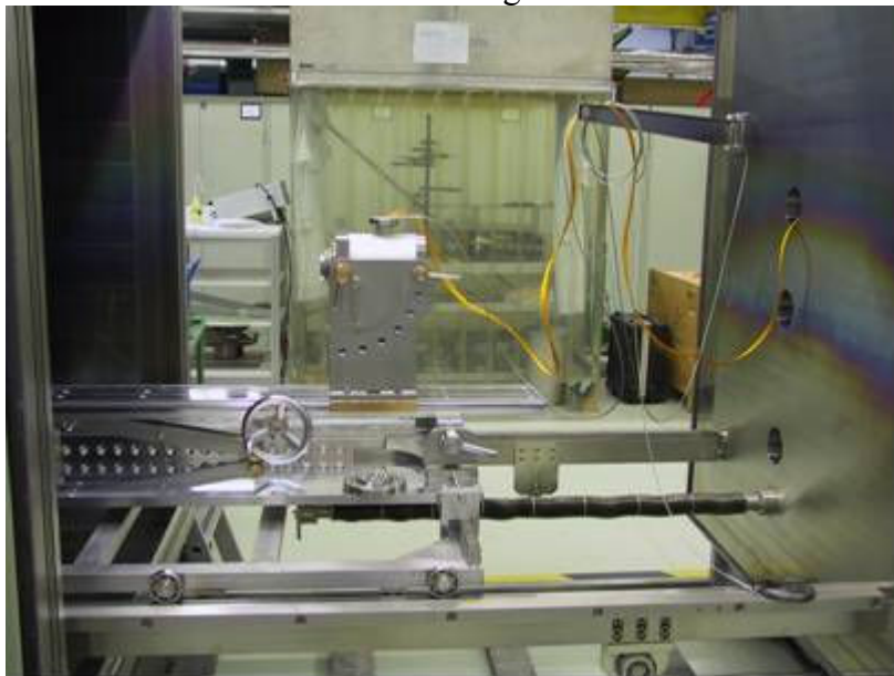
Figure JRA1.2.7: Motor box and current supply with Kapton© isolation
