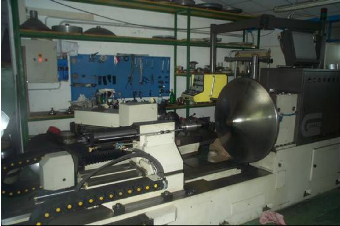
Figure JRA1.3.1: The spinning lathe used for the fabrication of seamless cavity prototypes. The lathe had only one turret which held the rollers.
