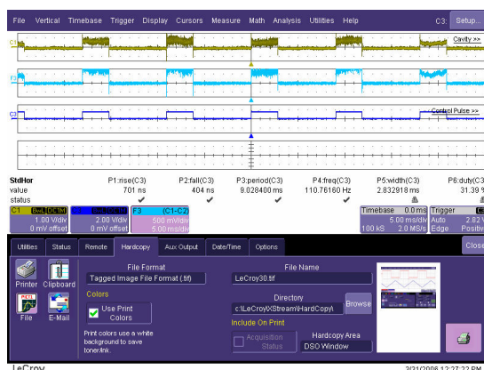
Figure JRA1.4.11: Traces recorded during test with the pulsed bias: the upper trace - the ion-current upon the cavity wall vs time (at bias -60V, repetition - 110 kHz, 31.5% duty); the middle trace - a differential current readout with noise filtering; the bottom trace – the bias voltage waveform.
