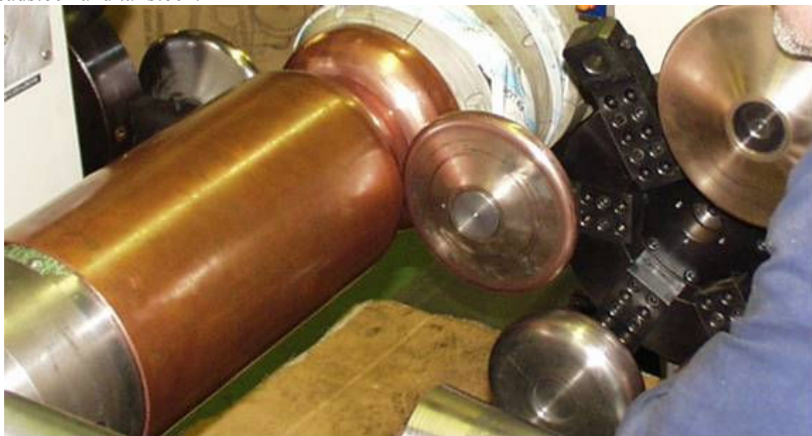
Figure JRA1.3.3: Phase of the double turret necking process during the spinning parameter definition action.
