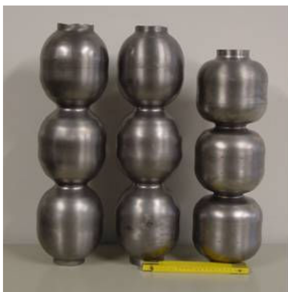
Figure JRA1.3.7: Example necking of the niobium three cell unit.
