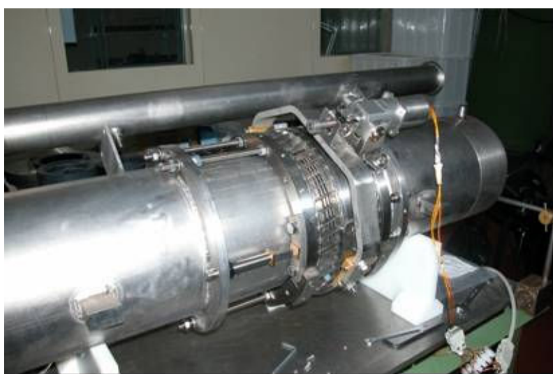
Figure JRA1.8.2: Complete assembly provided with leverage mechanism and stepping motor.
