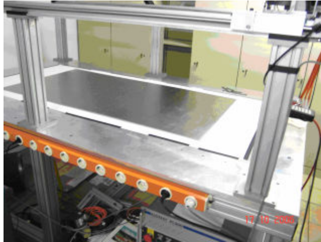
Figure JRA3.3.9: Eddy current testing of the sheets at ROHMANN company
