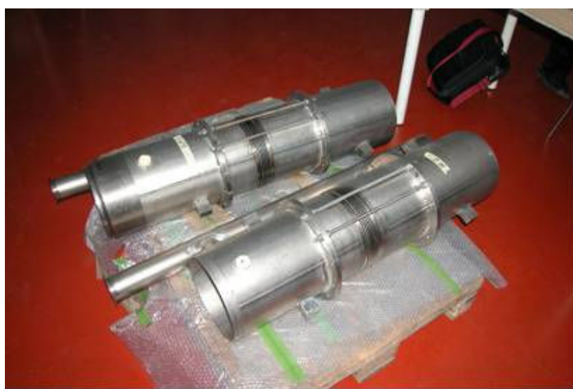
Figure JRA1.8.1: TTF cavities modified Helium tanks
