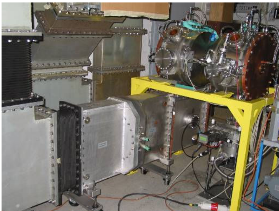
Figure JRA3.2.14: CCDTL pre-prototype at the high power test stand (waveguide side).
