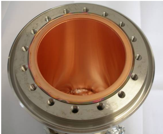
Figure JRA3.3.2: Copper plating of the outer conductor (left) Doorknobs with adaptors for RF measurements (right)
