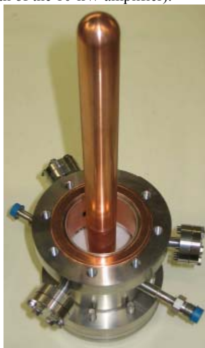
Figure JRA3.3.16: RF coupler with its antenna (left), test bench with the pair of couplers
