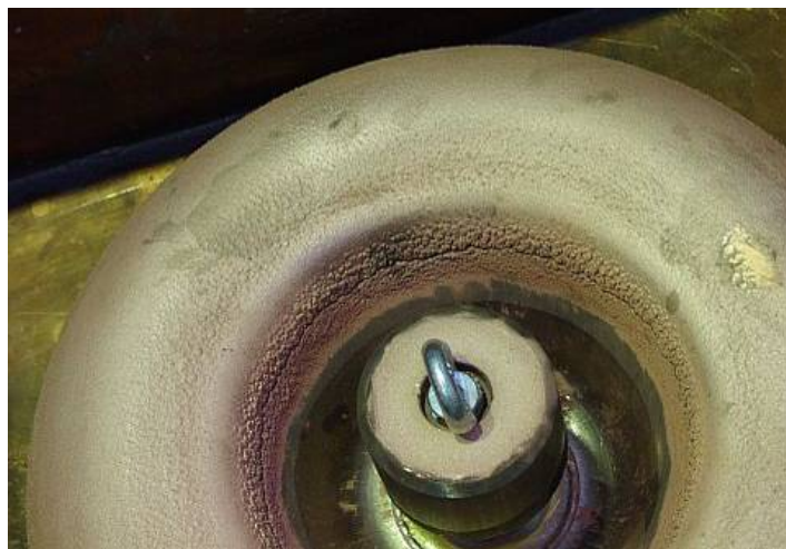
Figure JRA3.3.7: End cup as received from plasma spraying
