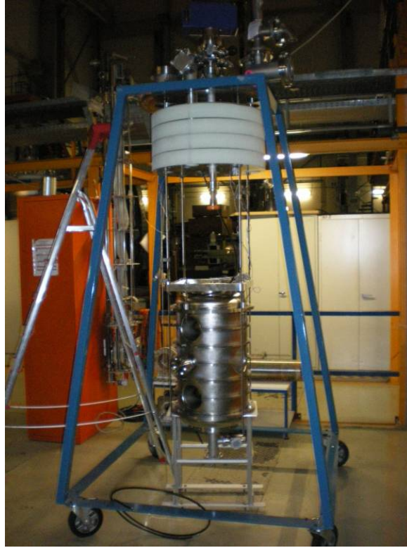
Figure JRA3.3.11: The 3-Spoke cavity in the cryostat frame at Juelich
