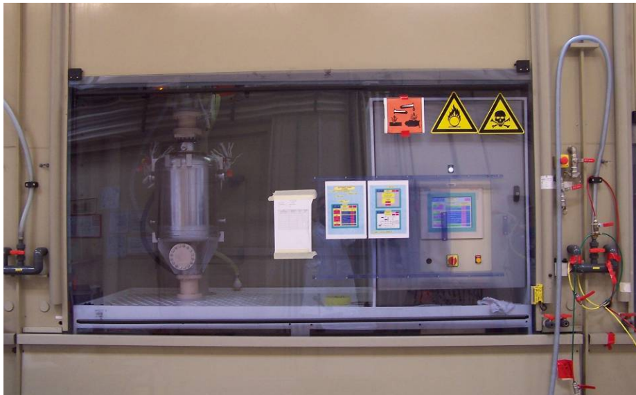
Figure JRA3.3.1: Chemical treatment of the Cavity B
