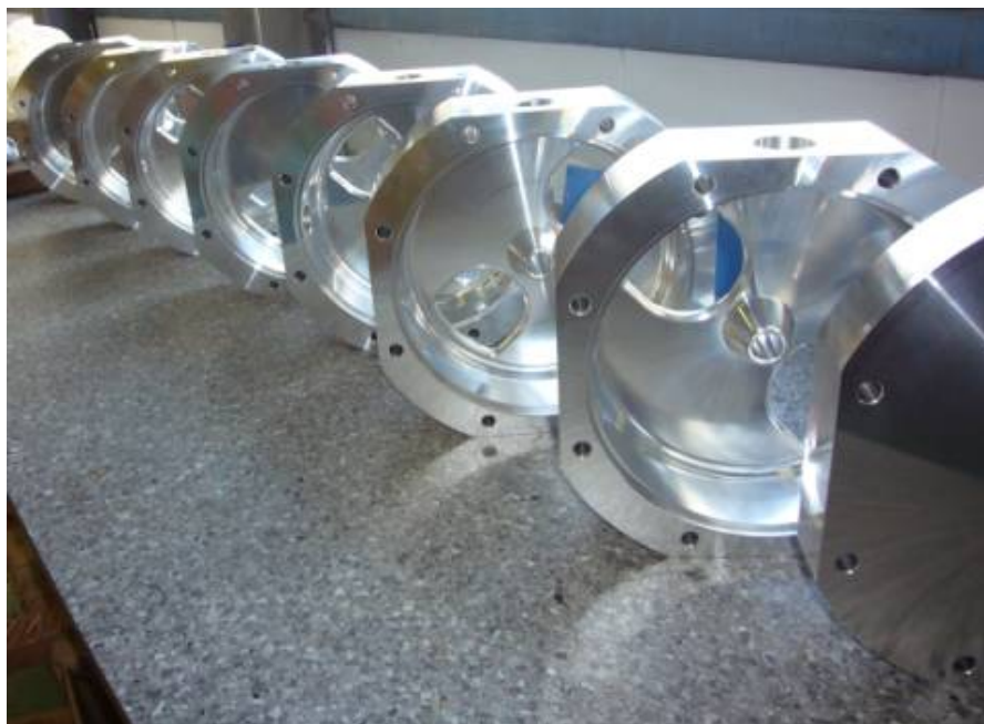
Figure JRA3.2.12: A 7 cell cold model of the PIMS.
