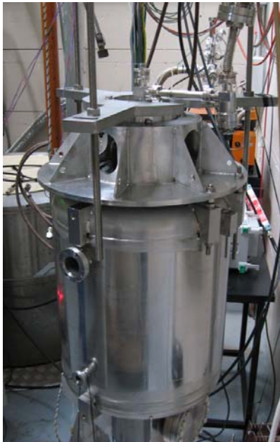
Figure JRA3.3.4: Cavity with helium tank and stiffening tube (left) Measurements of the surface resistance during RF test (right)
