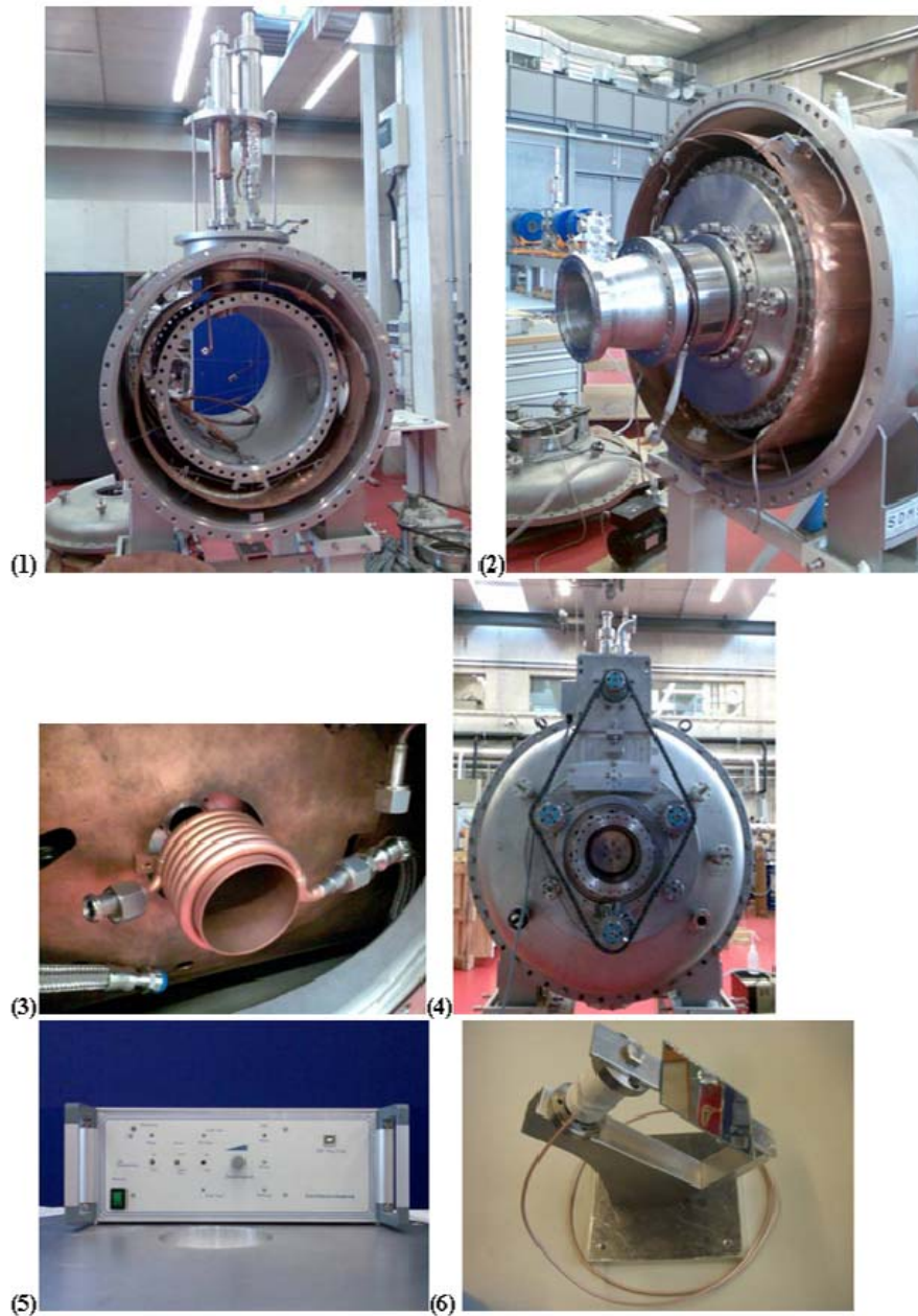
Figure JRA3.3.23: (1) The cryostat during alignment procedure (2) Beam lead-through including piezo retainer (3) Cooling loop at pump port (4) The slow mechanical tuner at performance check (5) The control unit of the mechanical tuner (6) Set-up for piezo frequency response measurement.
