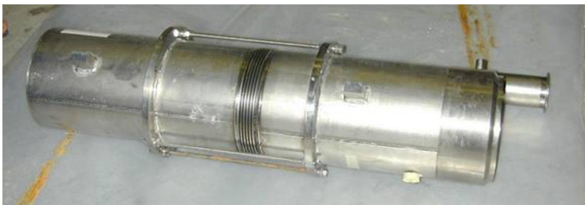
Figure JRA1.2.2: the modified He tank. The support screw rods, visible between welded rings, are temporarily placed to save the bellow from unwanted deformations.
