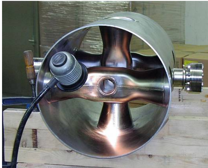
Figure JRA3.3.8: 352 MHz cavity with all spokes welded into the cavity body.
