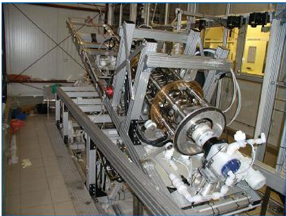
Figure JRA1.5.1: Picture on the DESY electropolishing equipment in the condition of dumping the acid after process ends
