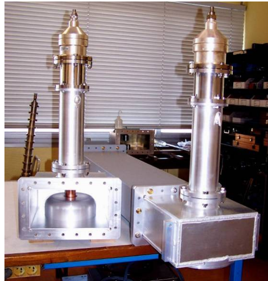
Figure JRA3.3.2: Copper plating of the outer conductor (left) Doorknobs with adaptors for RF measurements (right)
