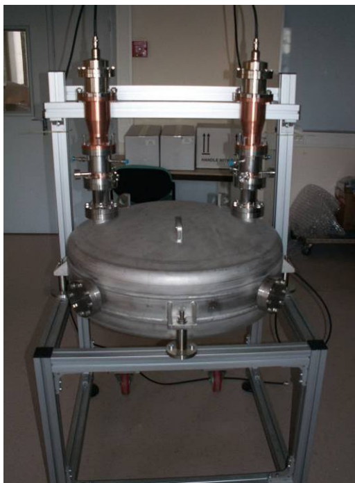
Figure JRA3.3.16: RF coupler with its antenna (left), test bench with the pair of couplers
