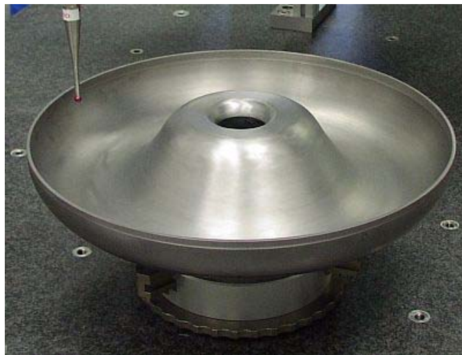
Figure JRA3.3.9: Niobium end cup on the precision measurement machine
