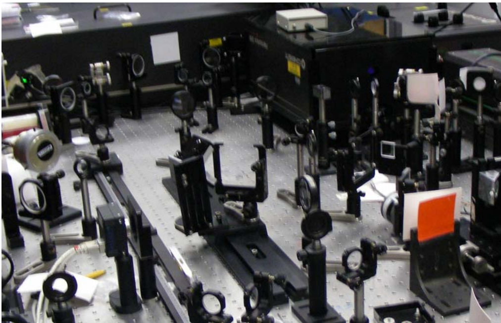
Figure JRA2.3.2: picture of the UV stretcher realized with transmission grating
