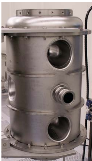
Figure JRA3.3.20: 3-Spoke prototype with its stiffeners
