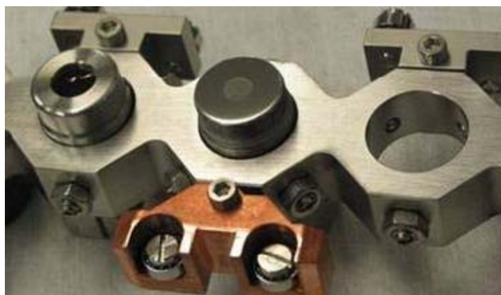
Figure JRA1.5.5: Cathode plug (in the center) in transport frame
