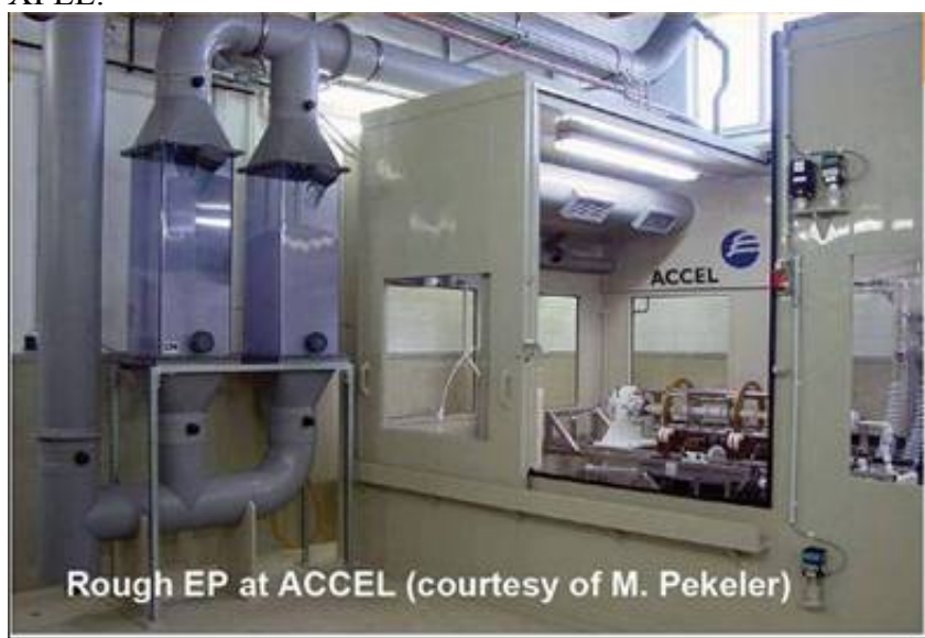
Figure JRA1.5.3: Industrialized EP set up at ACCEL Company in Bergisch Gladbach Germany
