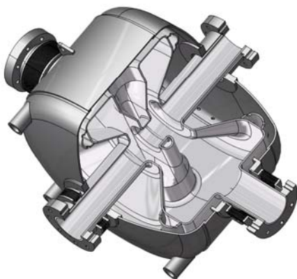
Figure 4.3.10: 2-gaps spoke cavity at Orsay
