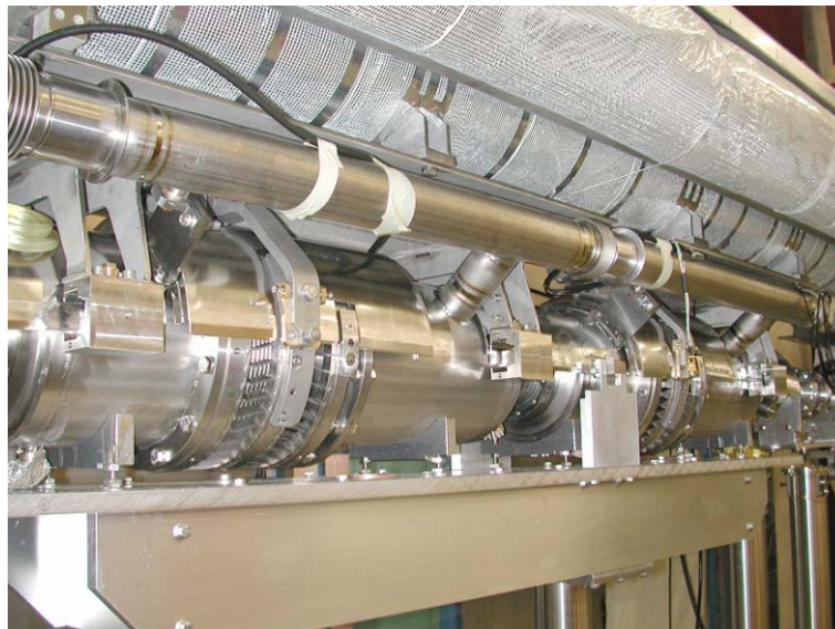
Figure 4.3.2a: Tuning system on a TTF superstructure
