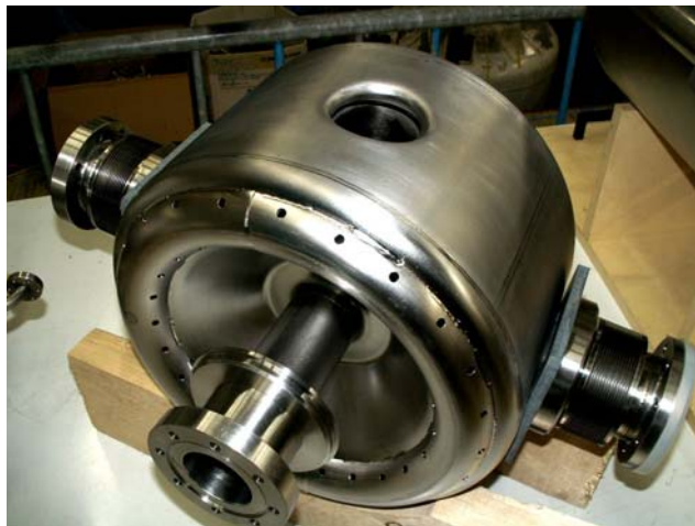
Figure 4.3.10: 2-gaps spoke cavity at Orsay
