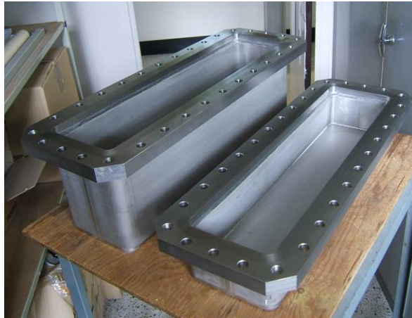
Figure 4.2.3: View of the two short-circuit wave guide terminations. They will be used to know the optimal position of the short circuit.
