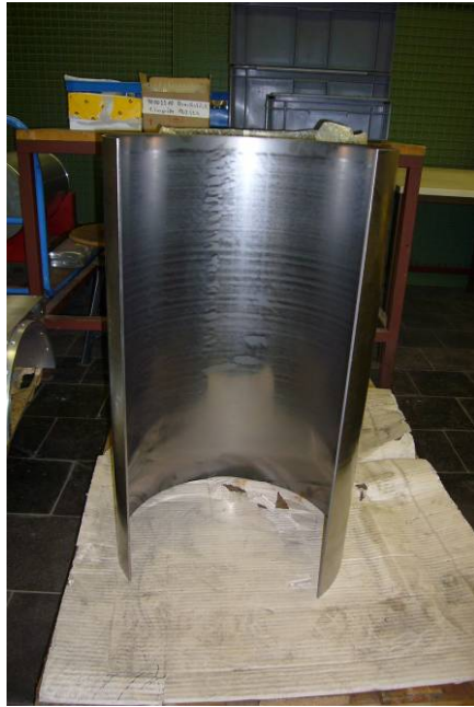
Figure 4.3.5: Rolled half shell of the cavity body (left) and coupler port with hot brazed SS flange (right)
