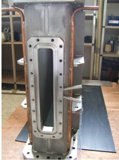
Figure 4.2.2: View of the water-cooled coupling window
