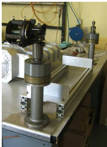
Figure 4.2.9: Preparation of the bead-pull measurement setup
