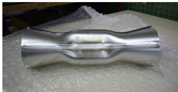
Figure 4.3.6: Formed niobium end cap (left) and welded niobium spoke (right)
