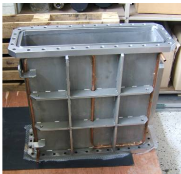
Figure 4.2.1: Side view of the coupling port and of its cooling system. The lateral flange (on the right) is the coupling window to the DTL tank.
