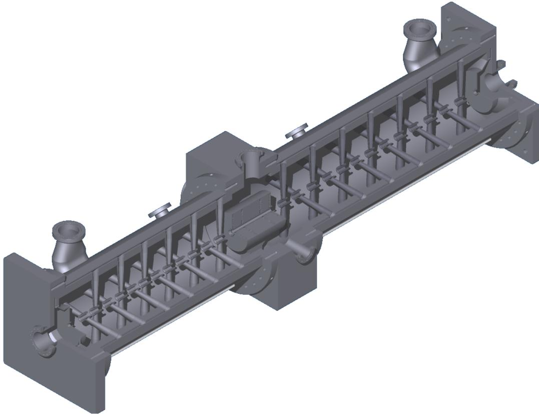
Fig.4.2.3: The second resonator of the FAIR proton injector
