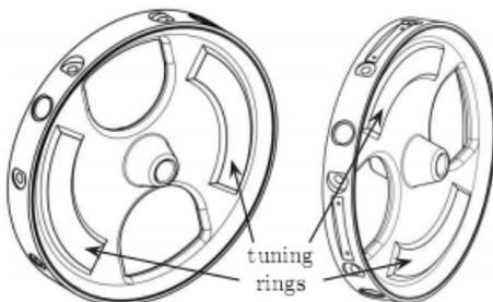
Figure 4.2.9: Tuning rings will be used to adjust the resonance frequency of each cell.
