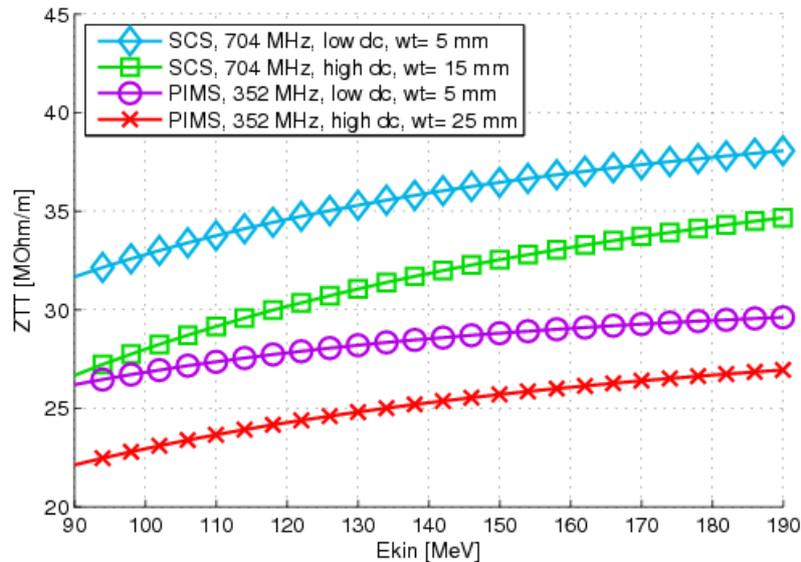
Figure 4.2.12: The effective shunt impedance per length in dependence of the particle energy for different accelerating structures and different duty cycles.
