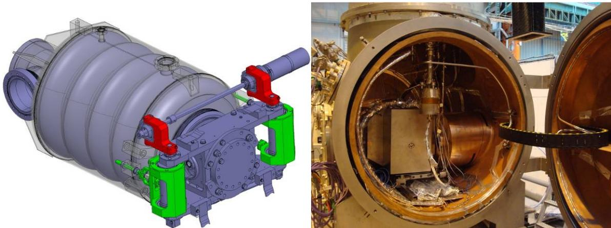
Figure 4.3.5 Cavity equipped with He tank and piezo tuner (left)
