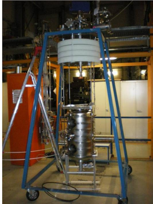
Figure 4.3.7 : The 3-Spoke cavity in the cryostat frame at Juelich
