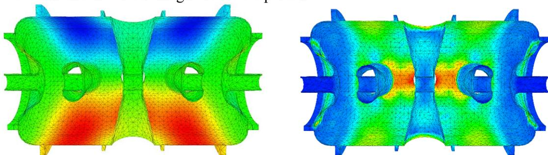
Figure 4.3.15: Deformation due to Lorentz forces (left)
