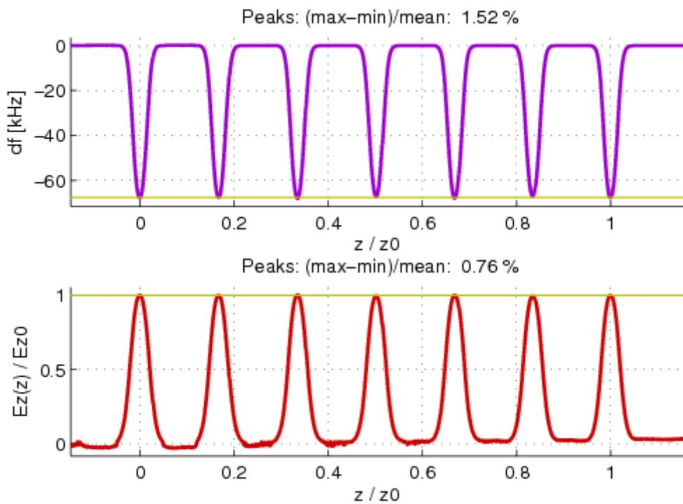
Figure 4.2.8: Bead pull measurement result of the 7 cell model. On the top, the frequency shift due to the perturbation induced by the bead, at the bottom the corresponding, normalised electric field along the symmetry axis.
