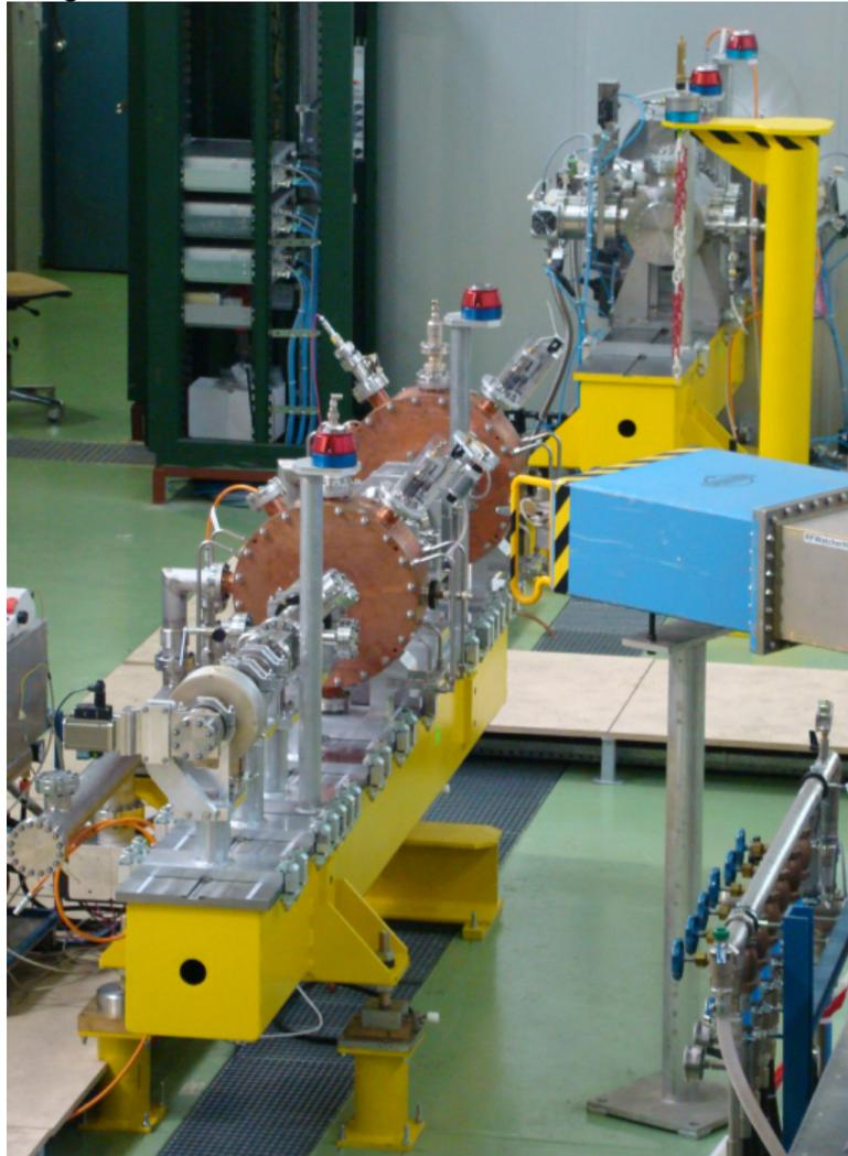
Figure 4.4.1 The CERN 3 MeV test stand line. In the background the H- source and LEBT assembly in progress; in the foreground the chopper line assembled and under vacuum.
