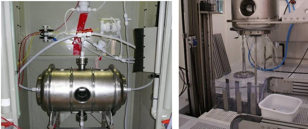
Figure 4.3.6 : Chemical preparation of the 3-spoke cavity at Saclay (left)
