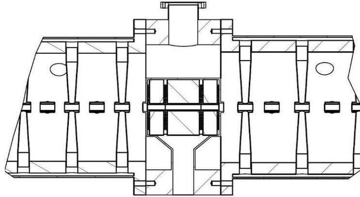
Figure 4.2.4: A detail of the coupling cell: the upper flange will be used as RF port
