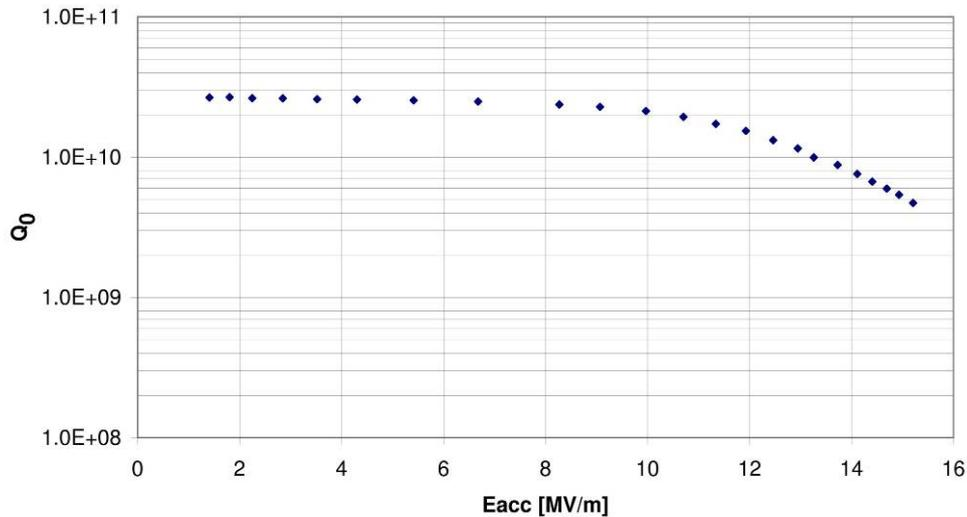
Figure 4.3.2 :  $Q_0/E_{acc}$  curve measured for the cavity B.
