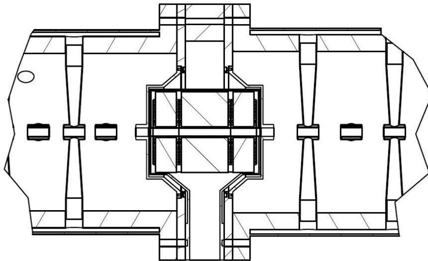
Figure 4.2.5: A detail of the intertank section between non coupled resonators
