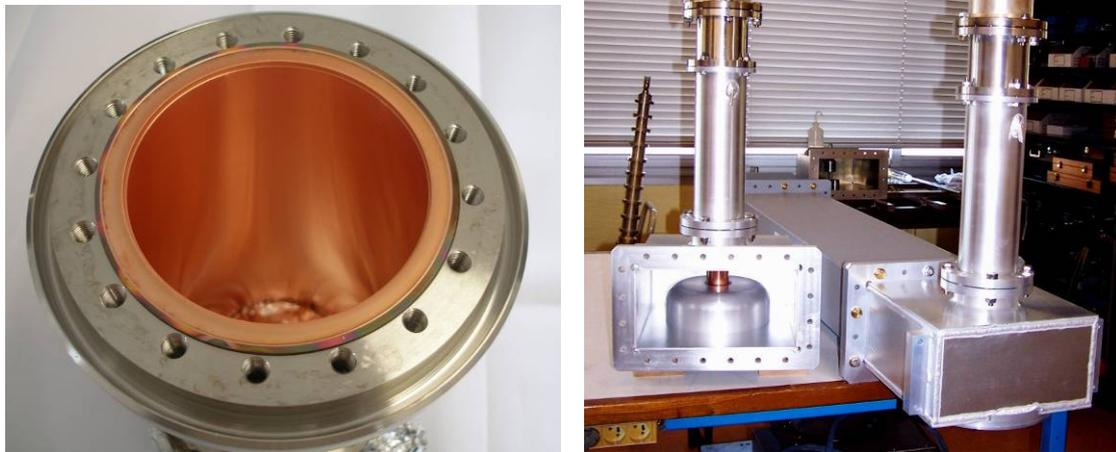
Figure 4.3.1 : Copper plating of the outer conductor (left)
