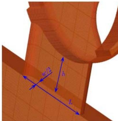
Figure 4.2.11: The wave guide coupler.  $L$  is the length,  $w$  the width and  $h$  the height of the coupling slot.
