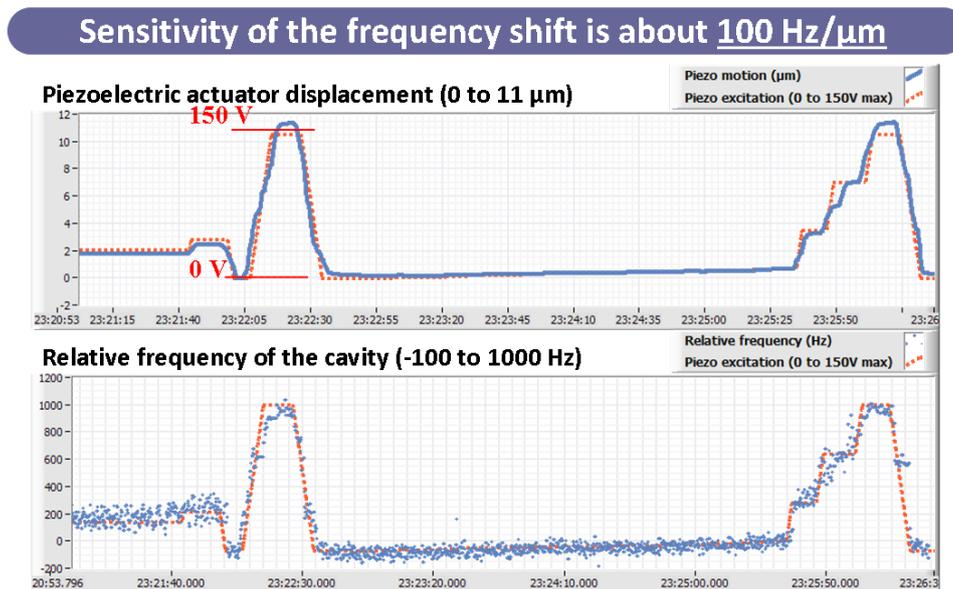
Figure 4.3.11 : Response of the cavity frequency while changing the piezoelectric length
