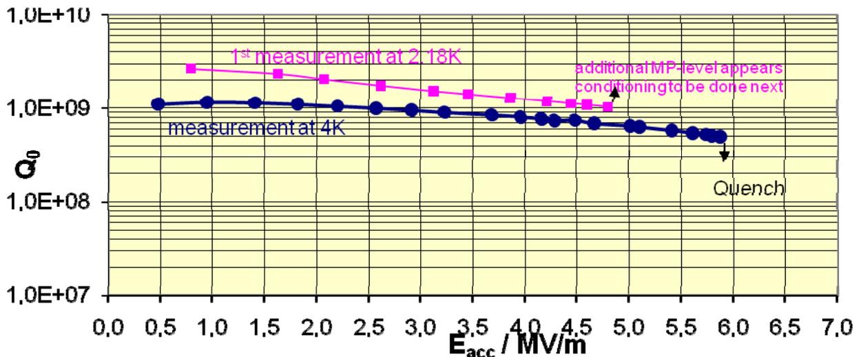
Figure 4.3.8 : First measurements of the 3-Spoke cavity
