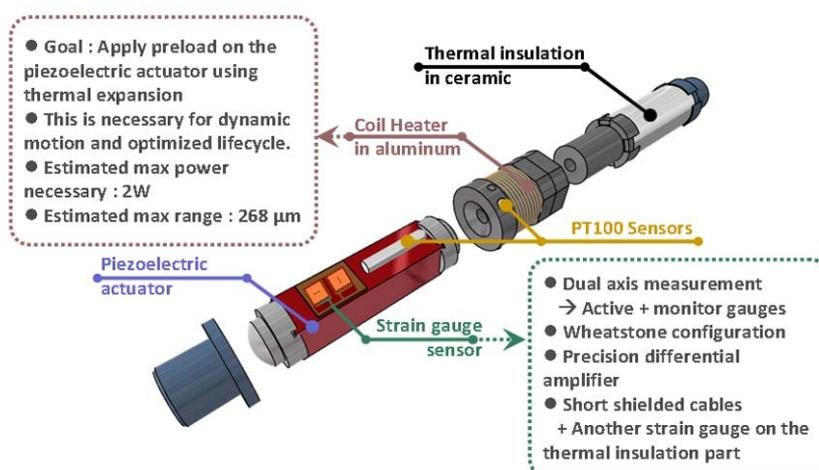
Figure 4.3.10 : Sketch of the piezoelectric set-up
