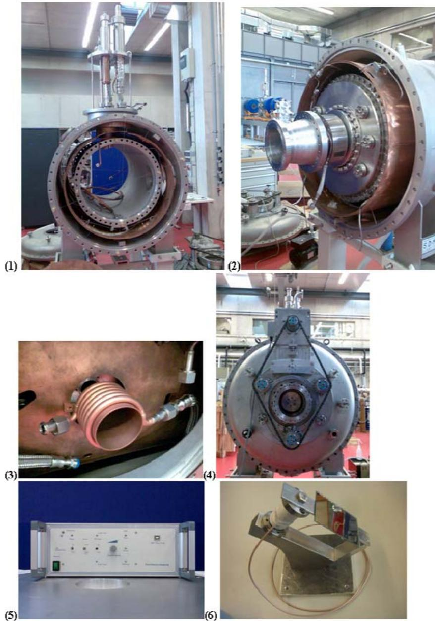
Figure 4.3.16 : (1) The cryostat during alignment procedure (2) Beam lead-through including piezo retainer (3) Cooling loop at pump port (4) The slow mechanical tuner at performance check (5) The control unit of the mechanical tuner (6) Set-up for piezo frequency response measurement.
