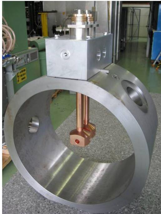
Figure 4.2.1: The CERN DTL pre-prototype structure.
