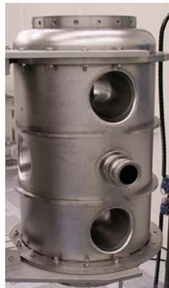
Figure 4.3.14: 3-Spoke prototype with its stiffeners
