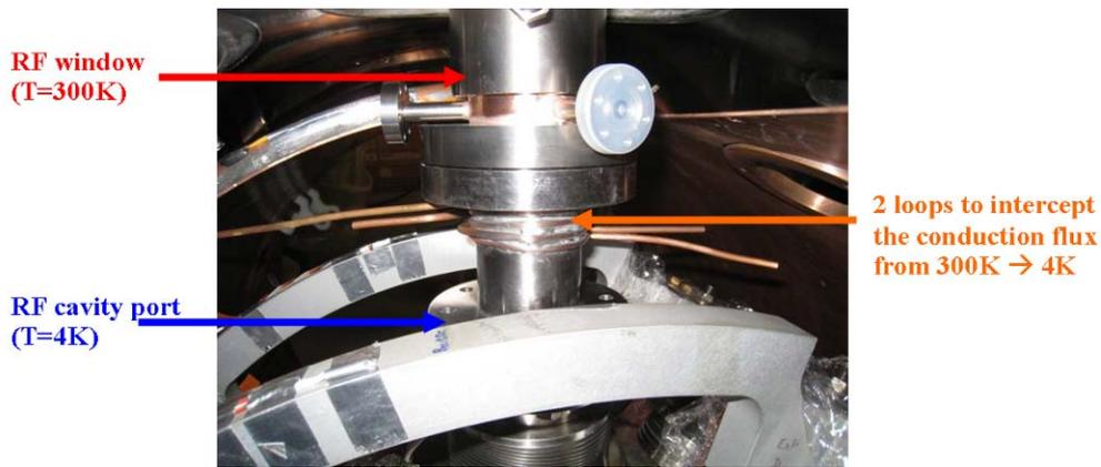
Figure 4.3.13 : RF coupler mounted on the spoke cavity
