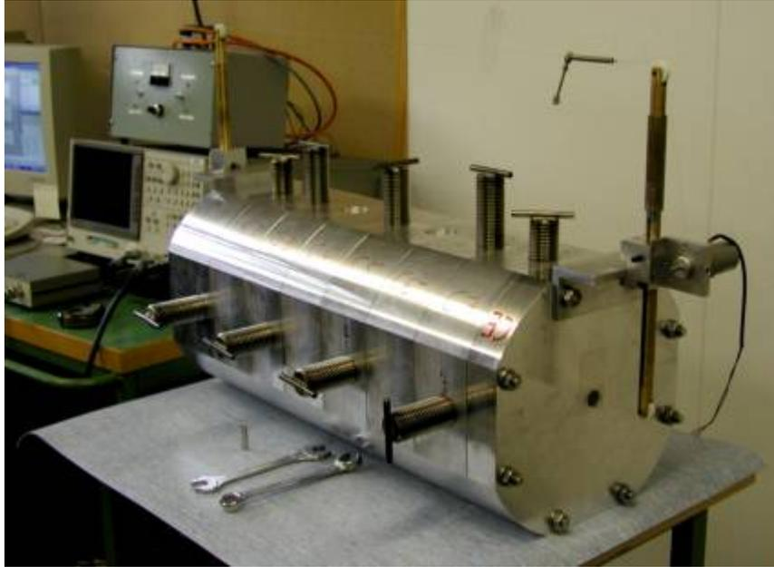
Figure 4.2.7: Bead pull measurement of a 7 cell PIMS module.
