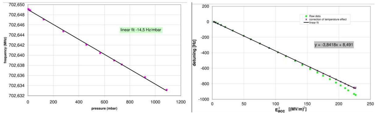
Figure 4.3.4 Helium pressure sensitivity measurements (left). Lorentz detuning measurements (right)
