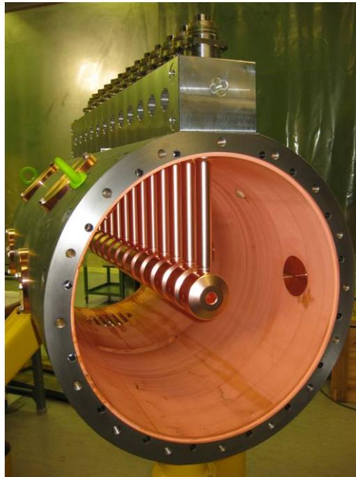
Figure 4.2.2: The assembled DTL prototype.
