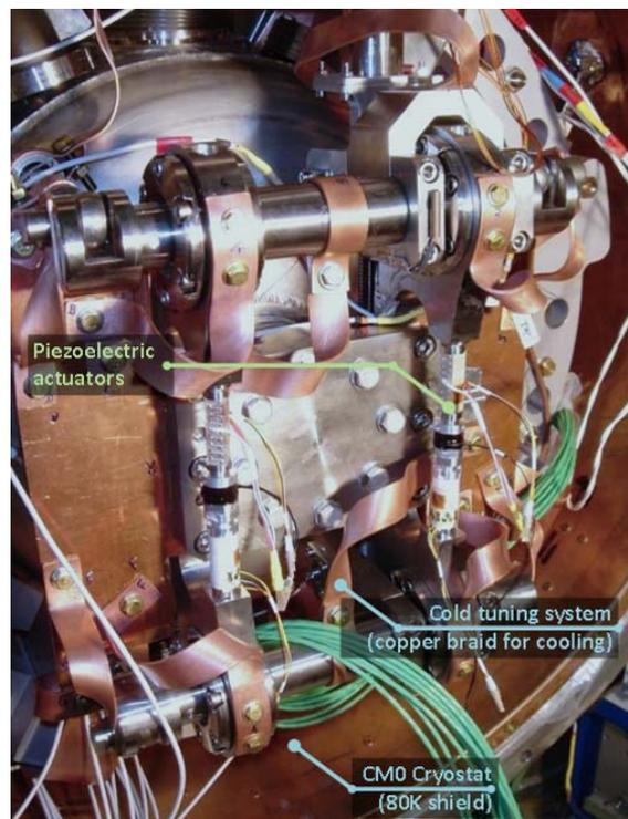
Figure 4.3.9: Tuning system of the spoke cavity with its piezoelectric-actuators
